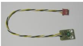
OSD current sensor with 20 cm wire.
